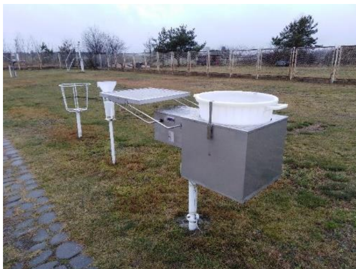
Figure 4.2 Automatic wet precipitation collector with open lid during precipitation, small precipitation collector for pH measurement in the background [photo by J. Biszczuk-Jakubowska].
