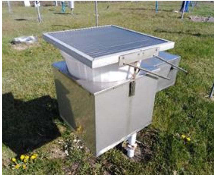
Figure 4.3 Automatic wet precipitation collector with the lid closed during no precipitation [photo: J. Biszczuk-Jakubowska].
